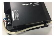
**PNote!** the power cord shall be fixed with bonding clamp in the kit, as shown in the fig.
