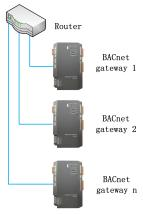
(2) Communication connection between BACnet gateway and AC units (n is the quantity of ODU system,  $n \le 16$ );
