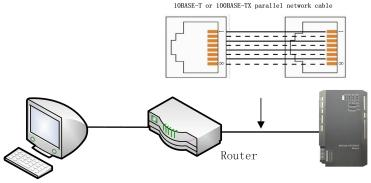
(2) Communication line connection between BACnet gateway and AC units:
