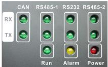
The above LED indicator is mainly consist of two parts: status indicator (run, alarm, power) and communication indicator (CAN, RS485, RS2332). The following table is the working status of each indicator.
